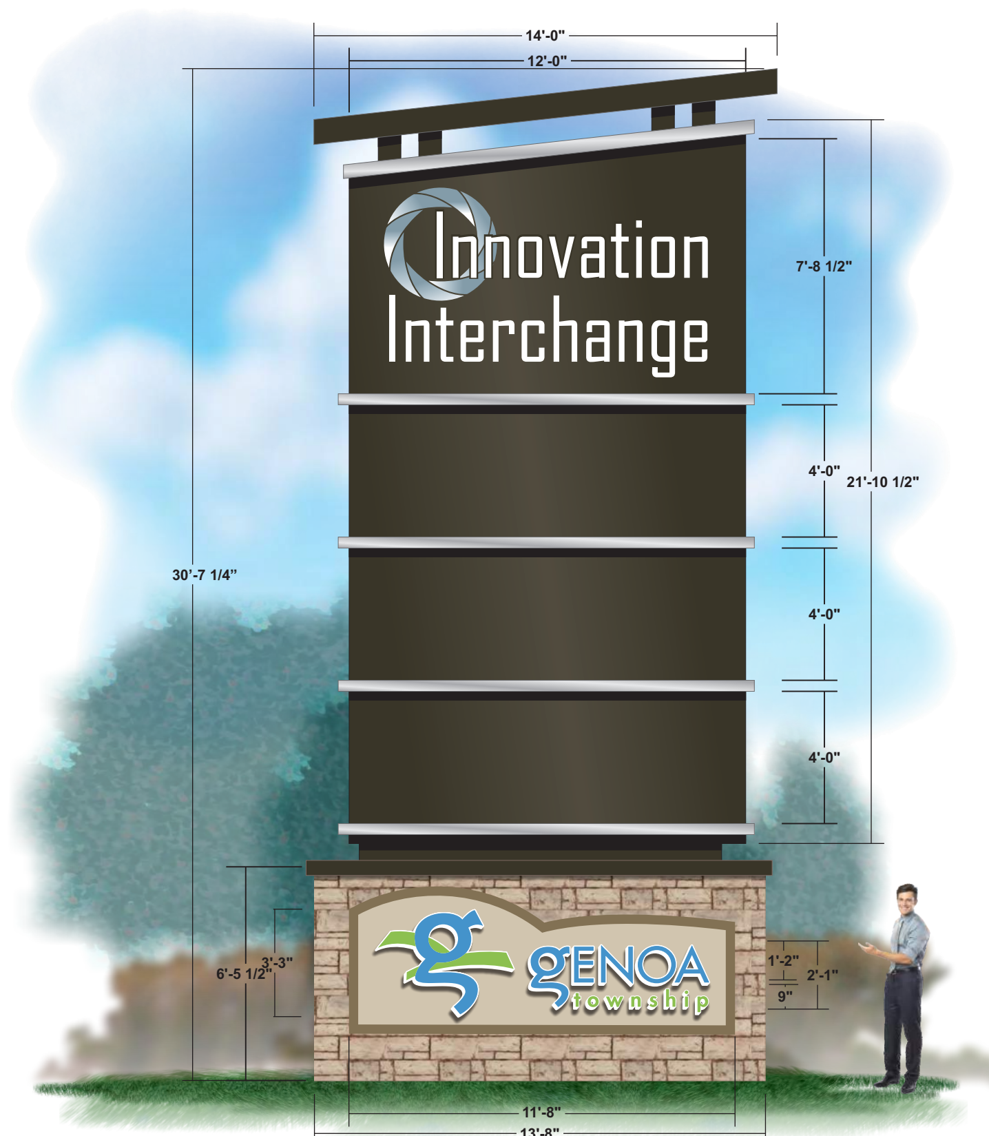
OPTION 1 CARVED & COATED HIGH DENSITY URETHANE FAUX STONE BASE FABRICATED DIMENSIONAL DIVIDERS SCALE 1/4" = 1'
