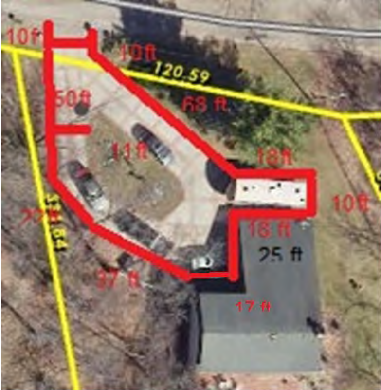
Figure 3. Parking dimensions. Dimensions are drawn on image.78 ft with 10 ft setback to street on one side with 18 ft* 10ft* 18 ft parking pocket where RV was parked next to garage. 10ft setback on the other side with 50 ft+22ft+ 37 ft+ 17 ft.
