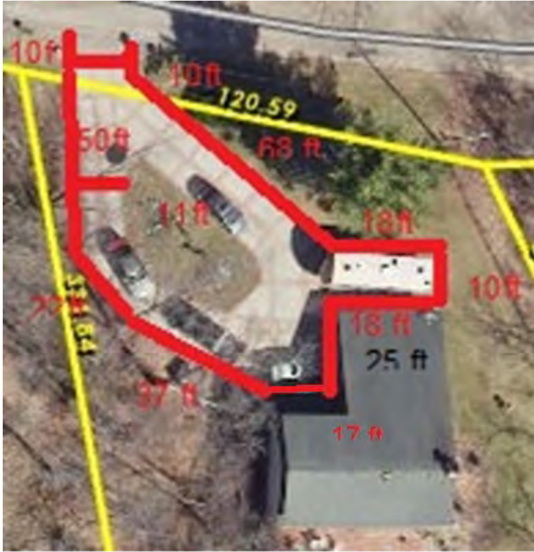
Figure 2. Parking dimensions. Dimensions are drawn on image. 68 ft+ 10 ft setback to street on one side with 18 ft* 10ft* 18 ft parking pocket where RV was parked next to garage. 10ft setback on the other side with 50 ft+22ft+ 37 ft + 17 ft.
