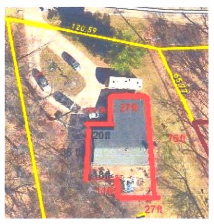
Figure 1. Building dimensions. 76 ft from front to back on long side, 11ft,36ft and 23 ft on the other long side, 47 ft on the short side of building.
