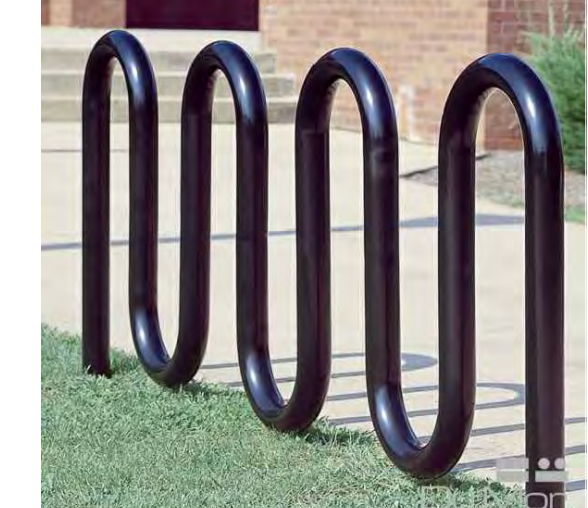
D bicycle rack (2-CONDITIONS) BIKE RACK BY DUMOR, INC. MODEL NO. 130-20 (S-2 SURFACE PLATE MOUNT) 2 3/8" O.D. BLACK POWDER-COATED LOOP OR EQUAL
