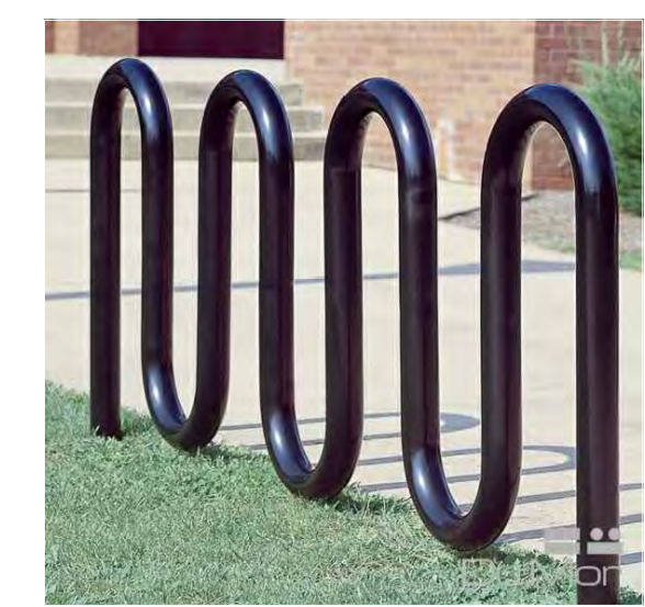
D bicycle rack (2-CONDITIONS) BIKE RACK BY DUMOR, INC. MODEL NO. 130-20 (S-2 SURFACE PLATE MOUNT) 2 3/8" O.D. BLACK POWDER-COATED LOOP OR EQUAL
