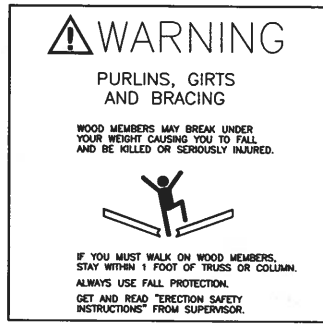
Wood Member Warning
