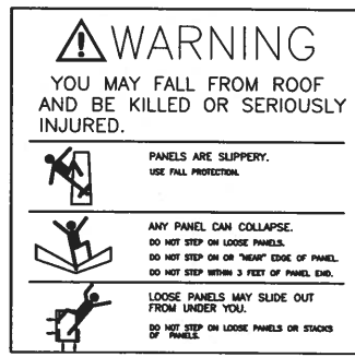
Roof Panel Warning
