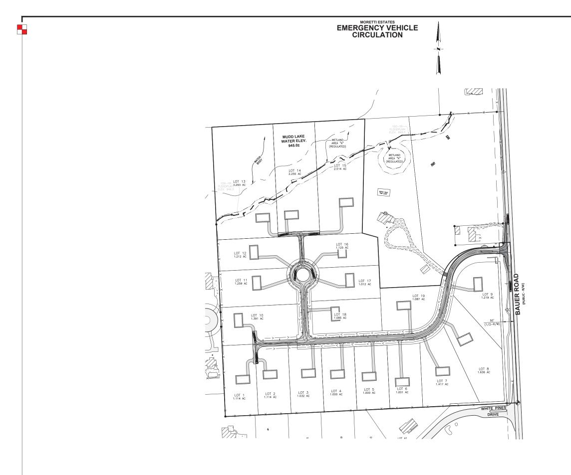
EMERGENCY VEHICLE 49.083 00 20.583' 4.667' 15.833 Brighton 49' Fire Truck Overall Length Overall Body Height Min Body Ground Clearance Track Width 49.083 8.167ft 7.500ft 8.167ft 5.00s 45.00° Lock-to-lock time Max Steering Angle (Virtual) FIRE TRUCK DETAIL CLIENT : EMERGENCY VEHICLE CIRCULATION
