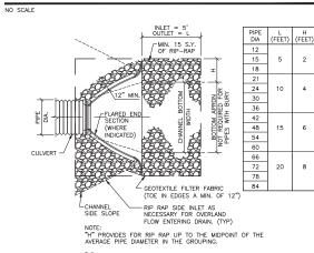
"L" FOLLOWS MINIMUM APRON LENGTHS BASED ON EMPIRICAL FORMULA U.S.E.P.A. 1976 L=30/D3/2 FOR TAILWATERS GREATER THAN 0.5D (D=DIAMETER).
