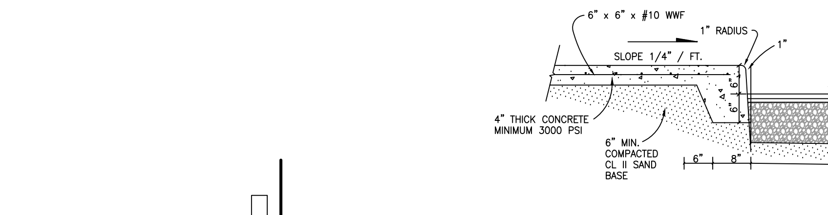
INTEGRAL CONCRETE WALK / CURB DETAIL (NO SCALE)
