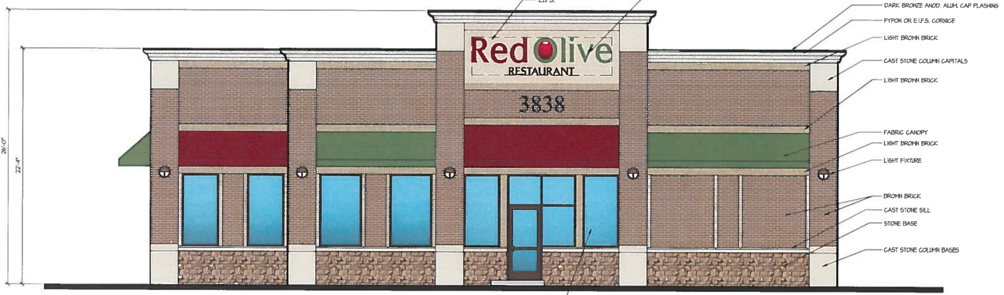
NORTH (FRONT) ELEVATION SCALE: 1/4" = 1'-0"
