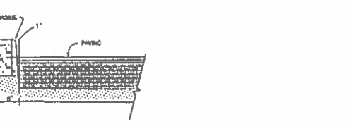
INTEGRAL CONCRETE WALK / CURB DETAIL (NO SCALE)
