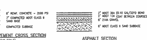
ASPHALT SECTION (NO SCALE)
