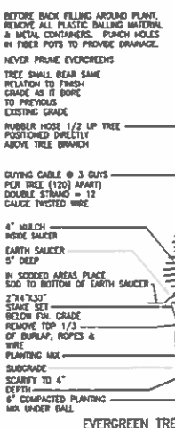
EVERGREEN TREE PLANTING DETAIL (NO SCALE)
