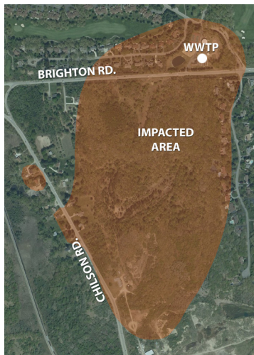
Figure 2: The area impacted by high sodium and chloride levels from the WWTP is shown in brown.
